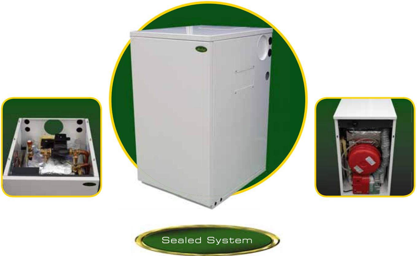
The Sealed System boilers are supplied with a 12 litre expansion vessel, pressure gauge, safety valve and automatic air vent. A circulating pump is also included in the boiler package which can be fitted within the boiler or remotely as required.
