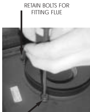
REMOVE FLUE RING
